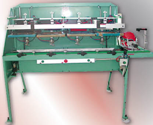
macchina semiautomatica a (4 colori) semi automatic silkscreen machine (4 colours)
